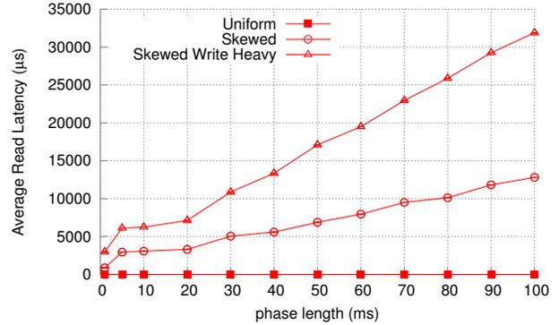
**Figure 13:** Average read transaction latencies in Doppel with the LIKE benchmark, varying phase length. A uniform workload, a skewed workload with 50% reads and 50% writes, and a skewed workload with 10% reads and 90% writes. 20 cores.
