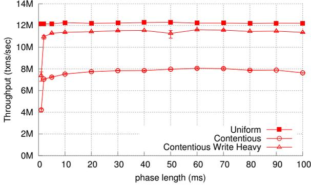
**Figure 14:** Throughput in Doppel with the LIKE benchmark, varying phase length. A uniform workload, a skewed workload with 50% reads and 50% writes, and a skewed workload with 10% reads and 90% writes. 20 cores.
