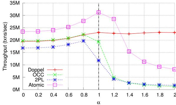
**Figure 11:** Total throughput for INCRZ as a function of  $\alpha$  (the Zipfian distribution parameter). The skewness of the popularity distribution increases to the right. 20 cores. The vertical line indicates when Doppel starts splitting keys.
