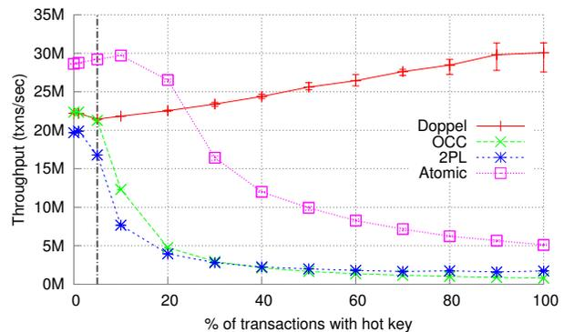
**Figure 8:** Total throughput for INCR1 as a function of the percentage of transactions that increment the single hot key, 20 cores. The vertical line indicates when Doppel starts splitting the hot key.
